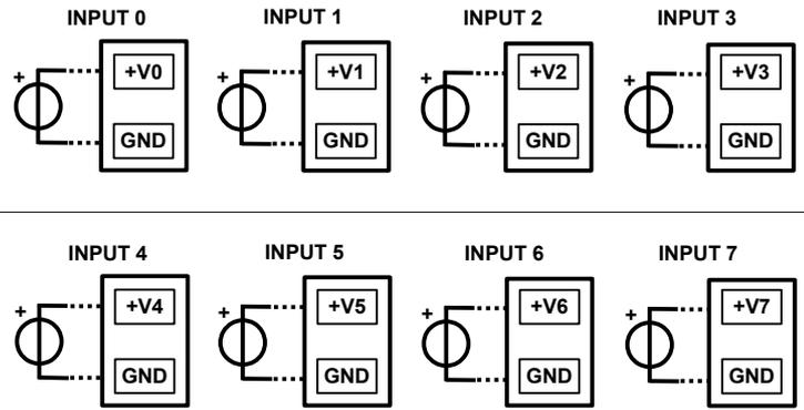
NOTE: the input channels are not isolated between them (terminal GND is common)
