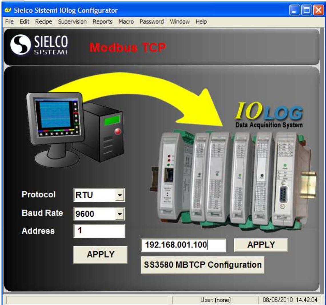
Configuring a module on Ethernet line (Modbus TCP)
