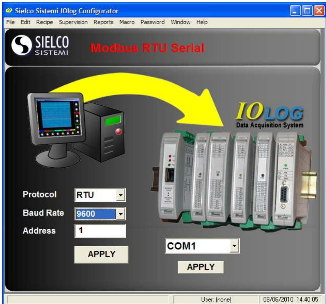
*Configuring a module over a serial line (Modbus RTU)*
