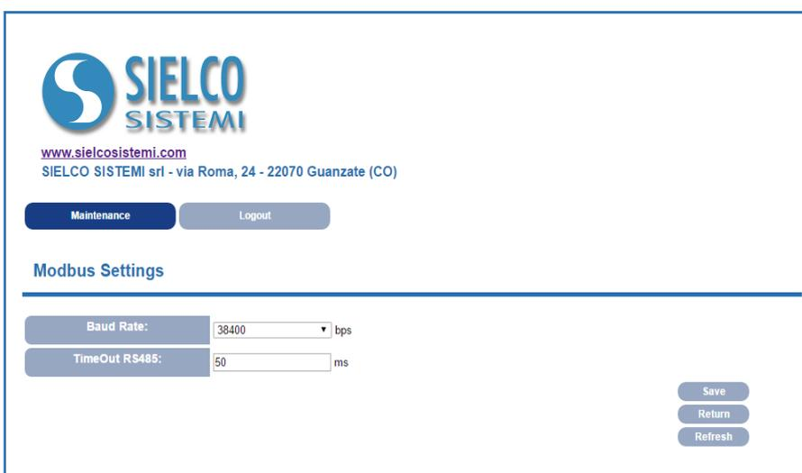
**Baud Rate:** through the drop-down menu set the Baud Rate of the RS485 port.
