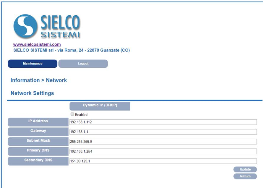
On this page it possible to change the TCP side settings (IP address, Subnet Mask, Gateway, DNS).
