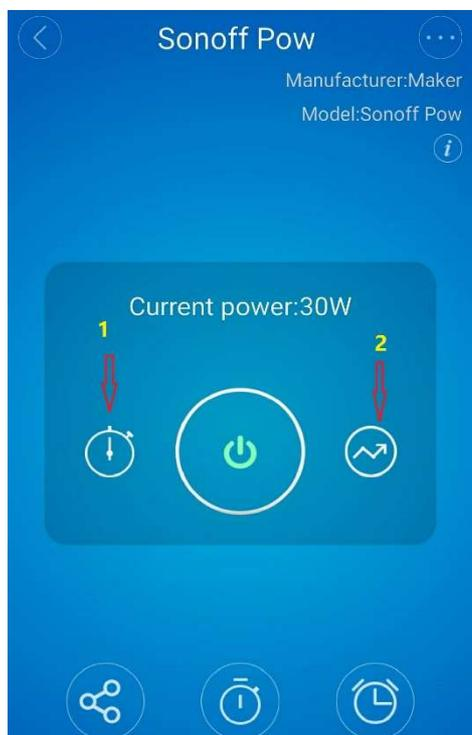
2. Tap 1 to measure device's power usage for a period of time. Tap "start" to count the power usage, and tap "stop" to stop counting.
