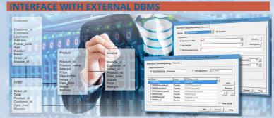
The "datalogger" function allows you to develop applications able to interface with any external DBMS accessible via ODBC (Mysql, ...), in order to record data tables. Thanks to a series of instructions (API) provided by the internal code, you can also interface the external DBMS through generic queries (SELECT, INSERT, UPDATE, ...) and read the results usable by the internal code routines. You can also directly interface with the external DBMS through the ODBC Client protocol.
